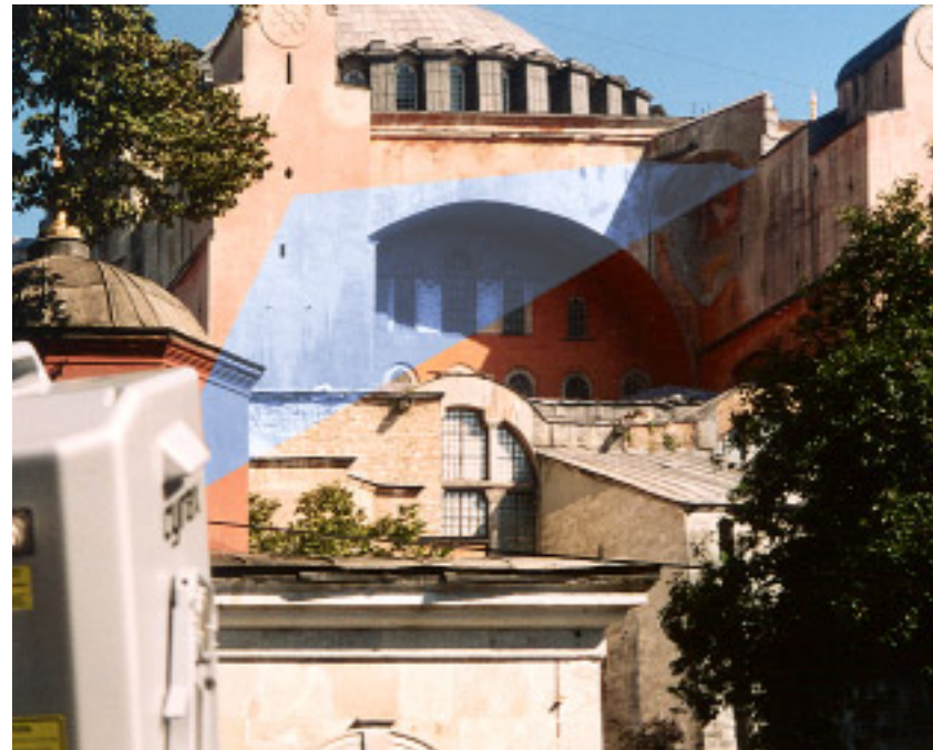
Laser beam deflection by two-axis mirror Range by light runtime
